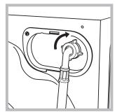
2. Connect the other end of the water inlet hose to the washerdryer, screwing it onto the appliance's cold water inlet, situated on the top right-hand side on the rear of the appliance (see figure).
